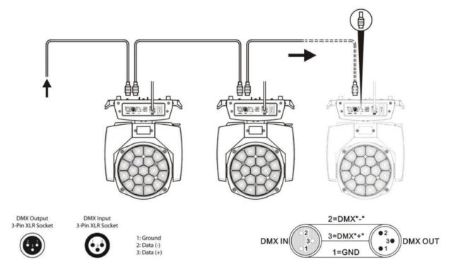
For installations where the DMX cable has to run a long distance or is in an electrically noisy environment, such as in a discotheque, it is recommended to use a DMX terminator. This helps in preventing corruption of the digital control signal by electrical noise. The DMX terminator is simply an XLR plug with a 120  $\Omega$  resistor connected between pins 2 and 3,which is then plugged into the output XLR socket of the last fixture in the chain. Please see illustrations below.
