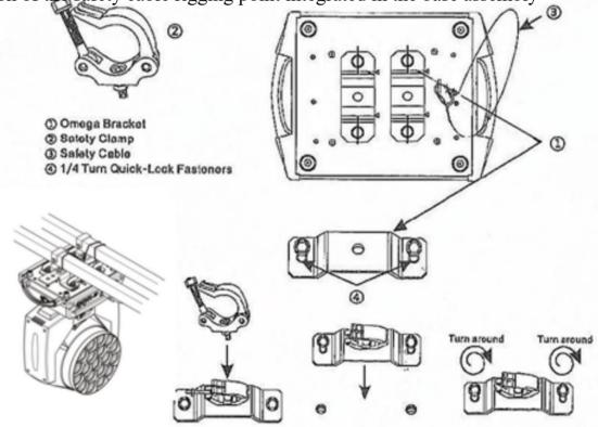
Regardless of the rigging option you choose for your 19pcs zoom, always be sure to secure your fixture with a safety cable. The fixture provides a built-in rigging point for a safety cable on the hanging bracket as illustrated above. Be sure to only use the designated rigging point for the safety cable and never secure a safety cable to a carrying handle.
